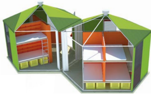
A hexagonal house being assembled (bottom) and in schematic (left and below). The design allows joining HaitiSOFTHOUSES to form a contiguous unit for families and extended families.
