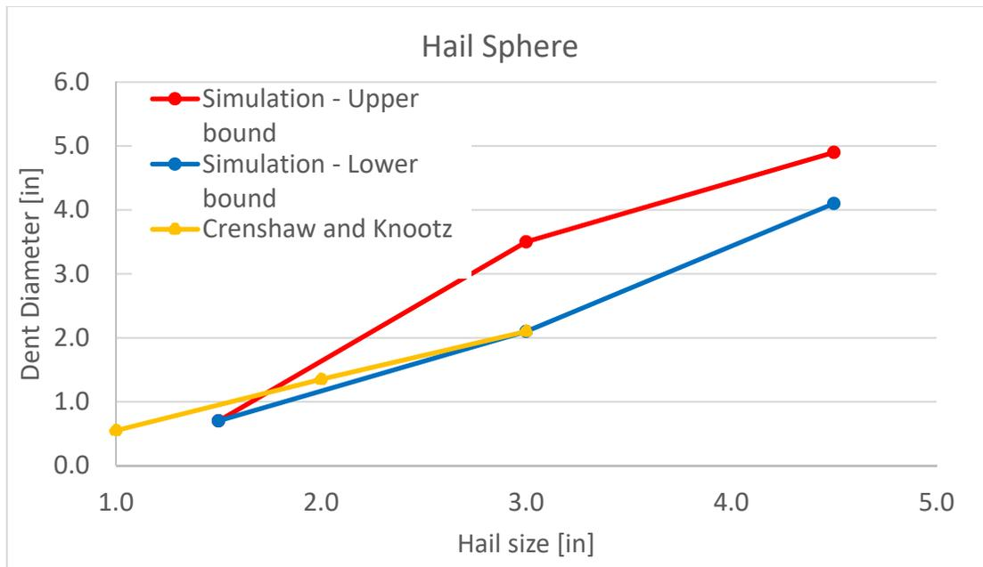
Figure 10: Dent diameter vs. hail size comparison between simulation (upper and lower bounds) and experimental data from Crenshaw and Knootz [8]
