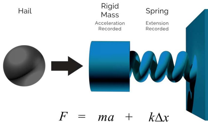
Figure 2: Validation experiment setup.
