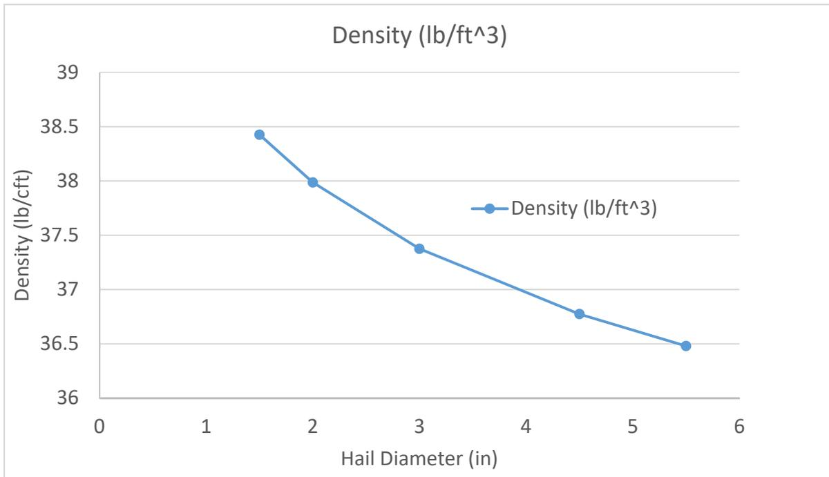
Figure 7 – Hail density vs. Diameter based on the data published in [6]
