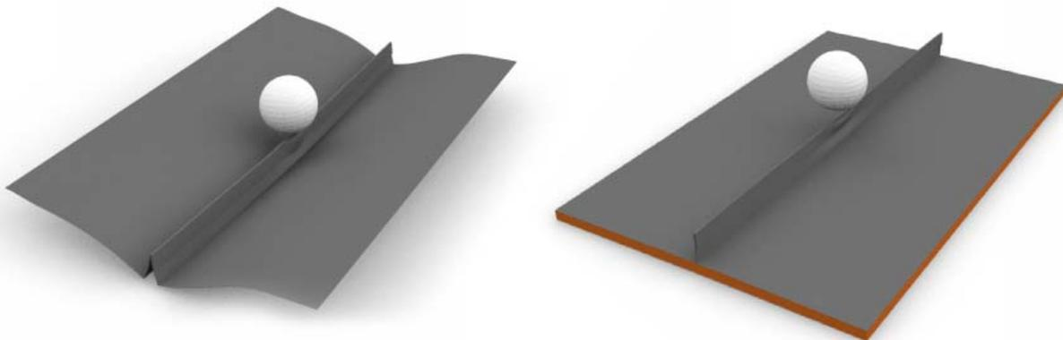
Figure 11: Simulated double-lock standing seam deformation due to hail impact
