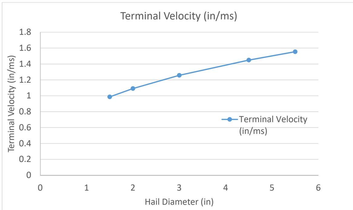
Figure 6 – Terminal velocity vs. Hail diameter based on the data published in [6]
