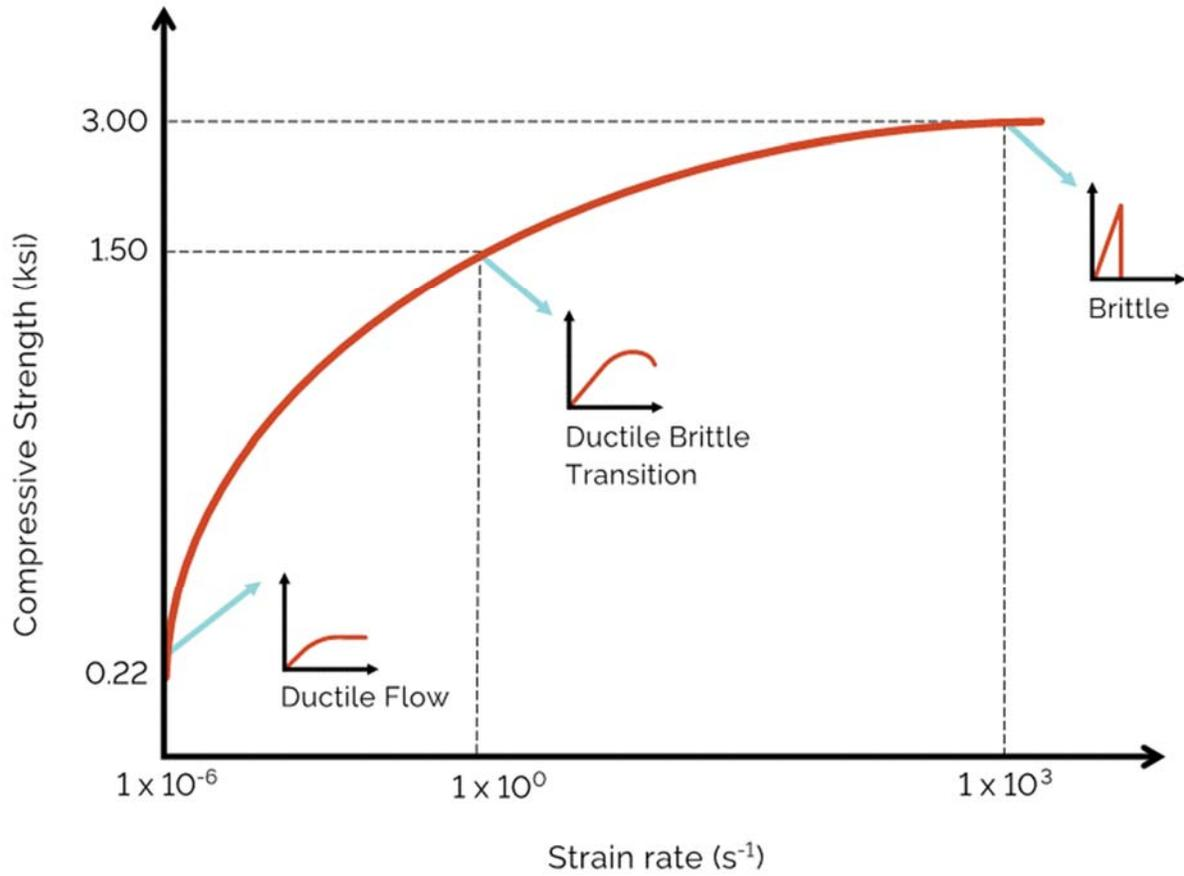
Figure 1: Rate dependence of ice mechanical response
