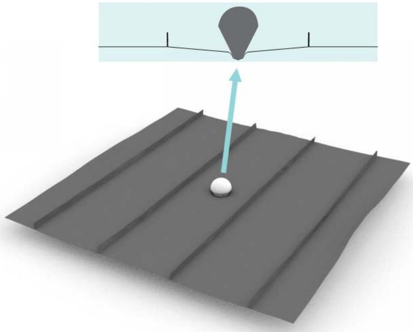
Figure 9: Deformed shape below 4.5 in hail cone
