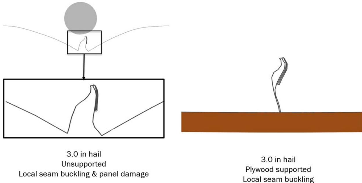
Figure 12: Section through double-lock standing seam deformed due to hail impact
