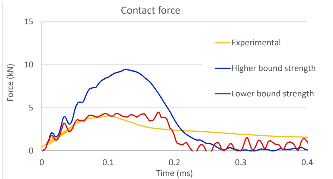
Figure 4: Contact (accelerometer) forces vs. time. Experimental in yellow, higher and lower bound strength simulated models in blue and red, respectively.
