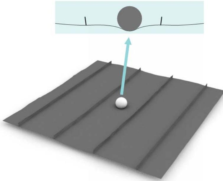
Figure 8: Deformed shape below 4.5 in hail sphere
